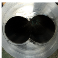
Bimetallic twin barrel for twin-screw machines
