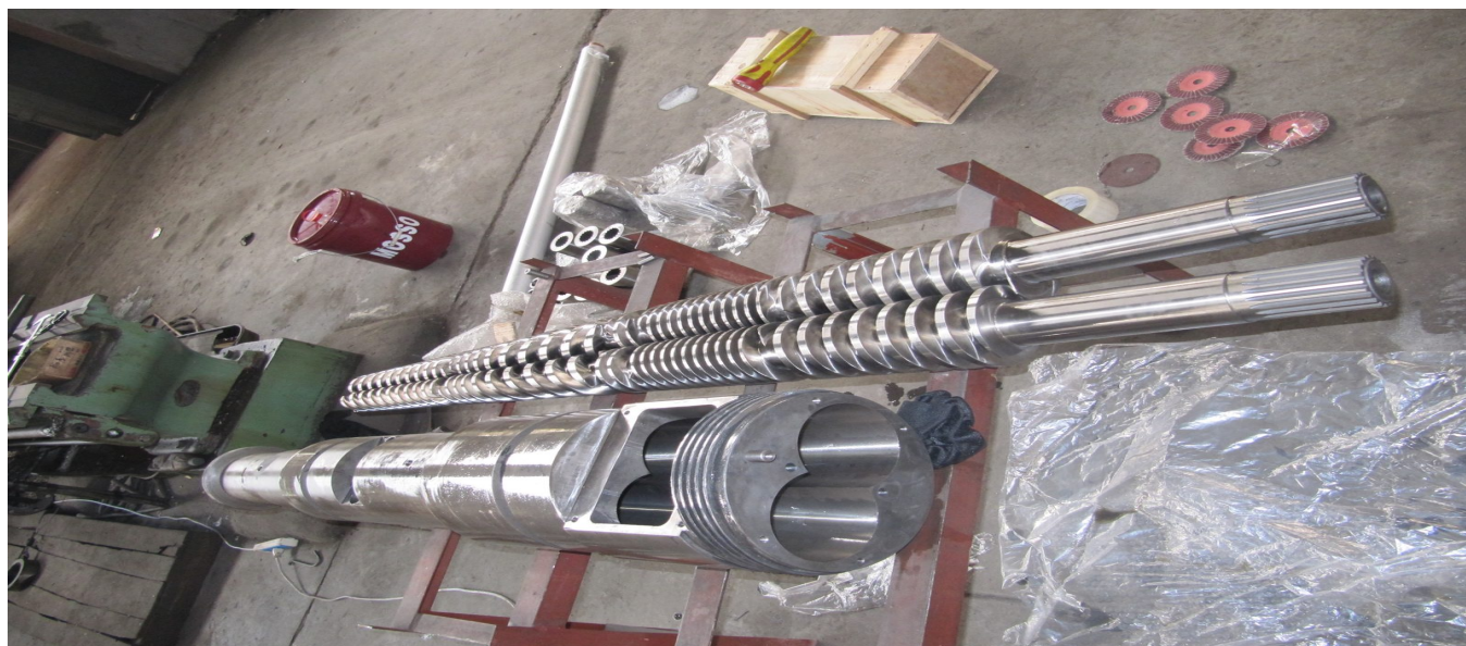
Screw & barrel sets on the shop floor of our 14,000 m2 workshop
